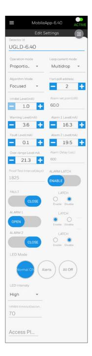
Enter a '**Detector ID**' (such as an equipment tag number), which can contain alpha numeric characters. Should the string entered contain invalid characters, a warning message will be displayed. Check the '**Detector ID**' and make changes where necessary.
