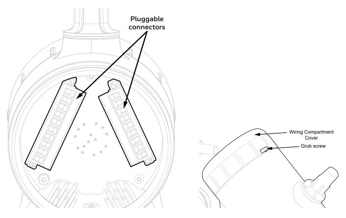
Figure 17. PCB Terminals
