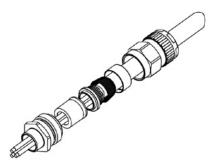
Figure 13. Example of cable gland
