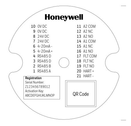
Figure 20. Terminal Connector Label
