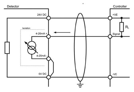
Figure 23. mA loop configuration as current sink
