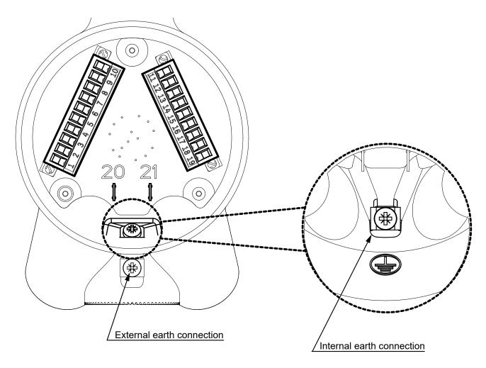
Figure 21. Terminal Wiring Compartment
