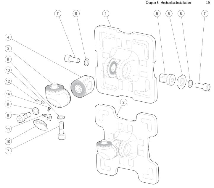
Figure 8. Universal Mounting Bracket exploded view
