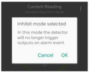
To return to Active mode, swipe the control in the top-right of the screen to the left and acknowledge the message.
