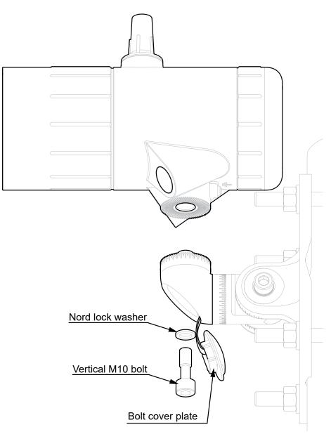
Figure 15. Detector attachment
