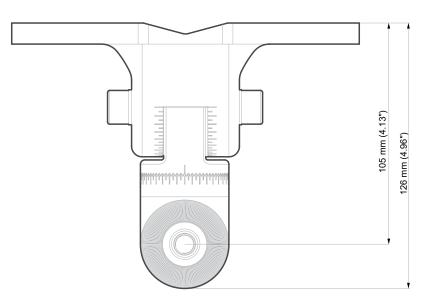
Figure 7. Universal Mounting Bracket general view and dimensions
