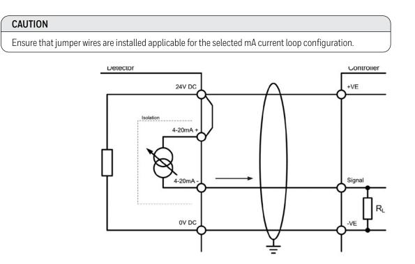
Figure 22. mA loop configuration as current source
