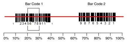
Scan **Centering On**, then scan one of the following bar codes to change the left or right of the centering window. Then scan the percent you want to shift the centering window using digits on the inside back cover of this manual. Scan **Save**. Default Centering = 40% for Left, 60% for Right.
