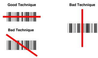
The best focus point for reading most code densities is about 5 inches (12.7 cm) from the unit. To read a single bar code or multiple bar codes (on a page or on an object), hold the scanner at an appropriate distance from the target, pull the trigger, and center the aiming beam on the bar code.
