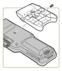
3. Lock the CK3/CK65 into place by lowering it into the IP30C locking bracket.
