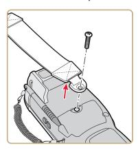
2. Attach the mounting plate onto the mobile computer using the provided screw.
