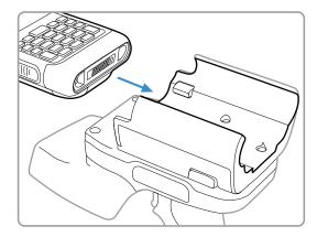
To remove the IP30C, press the two release latches (one on each side) and slide the unit out of the reader.
