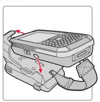
4. Lock the computer into place by angling it into the IP30C locking bracket.
