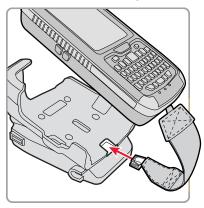
3. Lock the computer into place by lowering it into the computer mounting bracket.
