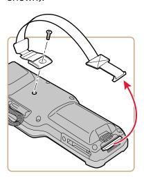
2. Attach the mounting plate onto the CK3/CK65 using the Phillips head screw provided with your IP30C. Turn the screw clockwise to secure the mounting plate onto the mobile computer.
