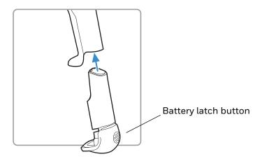
2. Push the battery latch button and slide the battery in until the battery is secure.
