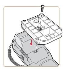
3. Lock the computer into place by angling the mounting plate into the IP30C locking bracket.
