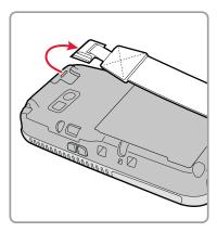
2. Insert the hand strap into the mounting bracket.
