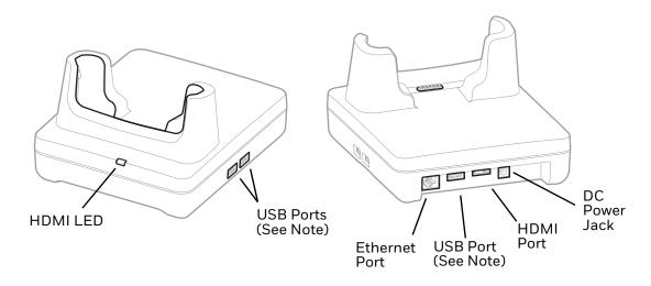
**Note:** The dock supports USB direct connections only. The dock does not support USB hub connections, including keyboards with USB port(s).
