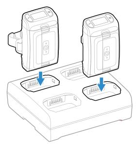
It is important that devices are inserted into the charging pocket correctly. Inserting the device incorrectly could result in damage to the device or the charger.
