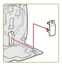
Insert the media sensor and cable assembly into the printer base and snap the sensor in place.
