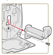
From the electronics side, push the media sensor cover out of the printer base and remove it.
