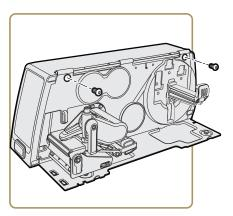
Use a T20 Torx screwdriver to remove the two screws located on the outside of the electronics cover.
