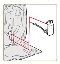
On the electronics side, connect the media sensor cable to the connector labeled "P26 Paper" on the main board.
