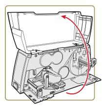
**2** Use the small wrench to loosen the nut that secures the media cover latches in place.
