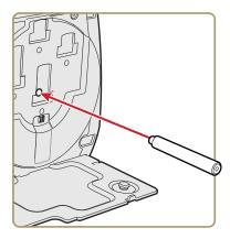
**6** Slide the oil-saturated felt washer and the reflective wheel onto the metal rod. Make sure the reflective side of the wheel faces the inside wall of the printer.
