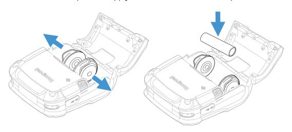
3. Insert the media through the external media opening below and through the printer.
