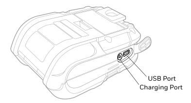
**Note:** Power off the printer before connecting a power or an interface cable.
