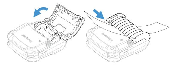
4. Press and hold the media button to calibrate the media sensor if required.
