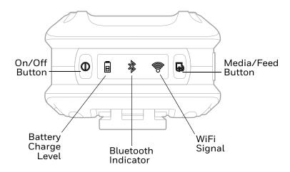
The front panel has an LED display and 2 buttons.
