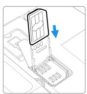
10. Close the holder with the card installed. Press down gently on the holder and slide it into the locked position.
