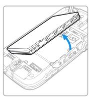
7. Lift up the edge of the SIM card access door (SIM 1 or SIM 2).
