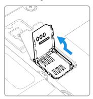
9. Insert the card in the holder with the contacts facing out.
