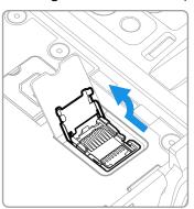
9. Insert the microSD card into the card holder with the contacts facing out.
