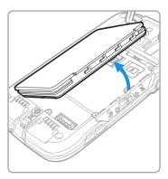
7. Lift up the edge of the SD card access door.
