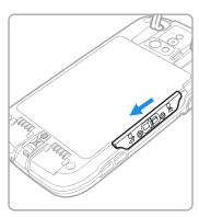
6. Lift up on the edge of the battery and remove it from the computer.
