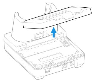
4. Insert the new cup tilted slightly towards the front of the base.
