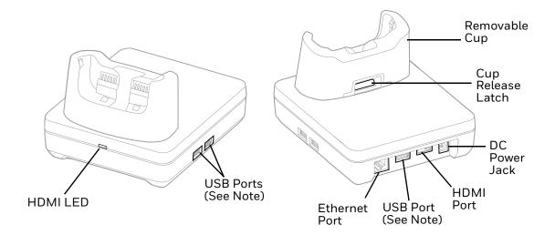
**Note:** The display dock supports USB direct connections only. The dock does not support USB hub connections, including keyboards with USB port(s).
