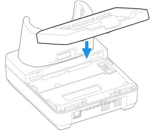
5. While holding the latch to the right, push the back of the cup into the base until it snaps in.
