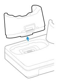
4. Insert the new cup tilted slightly towards the front of the base.
