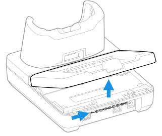
3. Release the latch and lift the old cup out of the base.
