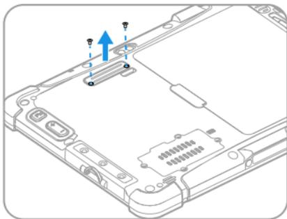
3. Install the reader using the screws provided.
