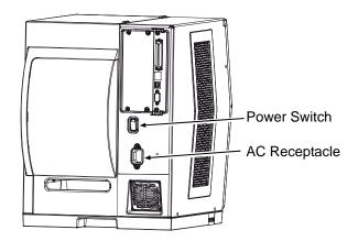
B) Remove the two Screws that secure the Back Panel to the Card Cage, and then remove the Back Panel.
