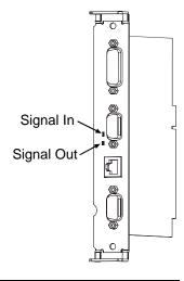
Input Monitor – Display incoming GPIO binary signal states using the ADVANCED MENU → DIAGNOSTICS → OPTIONS TESTING → TEST GPIO → MONITOR GPIO INPUT selection.
