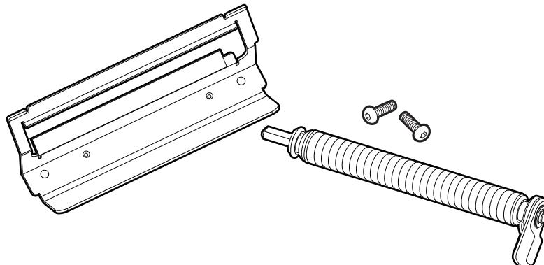
Before you install the linerless roller for the first time, you need to clean the roller and the printhead. Repeat the cleaning process every time you load a new roll of media. To clean the linerless roller and printhead, you will need:
