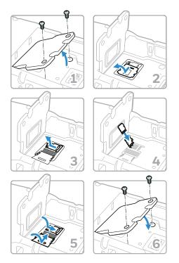
Note: Always place the computer in hibernate mode and remove the battery before attempting to install or remove a card.
