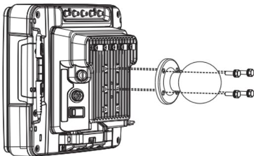
3. Attach VM1A assembly to RAM base using RAM arm and tighten knob on RAM arm.
