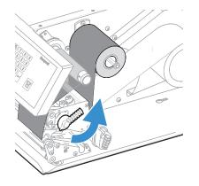
4. Remove any empty core from the media supply hub.
