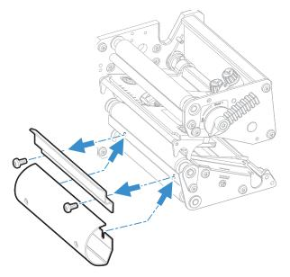
7. If you are using a media roll with a 76 mm (3 in) core, fit an adapter on the media supply hub.
