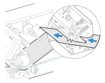
11. Pull out approximately 40 cm (15 in) of labels and remove the labels from the liner.
