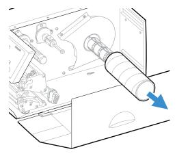
6. If your are using a media roll with a 76 mm (3 in) core, fit an adapter on the media supply hub.
