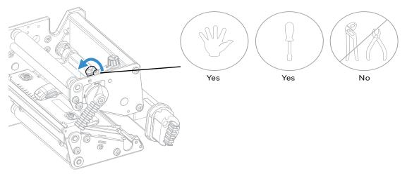
5. Move the pressure arm inward or outward until the arrow on the tip of the arm is centered with the media.
