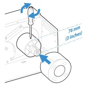
7. Fit a new roll of media on the supply post and push the roll in as far as it will go.
