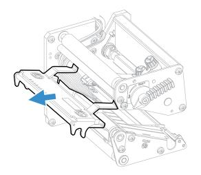
8. Disconnect the cables from the printhead. Note the snap-lock on the inner connector. Pull at the connectors, not at the cables.
