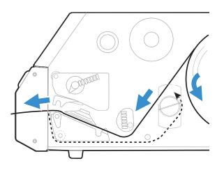
14. Turn the printhead lift lever clockwise to lower the printhead.
