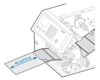
12. Route the labels around the guide plate and back under the print unit to the take-up hub.
