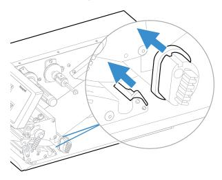
13. Route the media through the cutter between the two guide plates.
