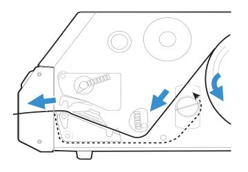
14. Turn the printhead lift lever clockwise to lower the printhead.
