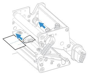
6. When the pressure arm is centered, tighten the knob to secure the arm. **Do not over-tighten the knob**.
