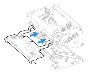
10. Connect the hooks of the printhead bracket to the headlift shaft. Make sure that the cables are not in the way.
