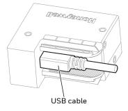
3. Secure the cable to the module using the slider:
