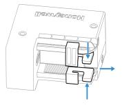
2. Connect a standard USB cable (standard USB-A to micro USB) to the module.
