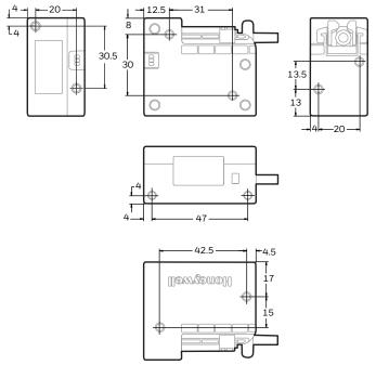
Units are in millimeters. Tolerances ±0.5 mm.
