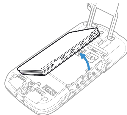
Sample battery removal, from CT60 mobile computer.
