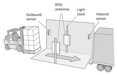
**Simple Portal System:** Arrow shows path for outgoing pallet. Accessories not to scale. Cables and reader omitted for clarity.
