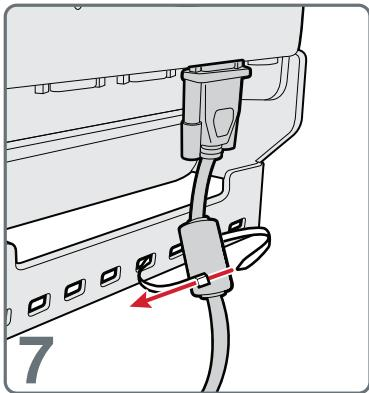
Optionally, use the mounting bracket to secure the cable from a large keyboard.
