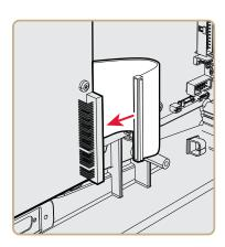
**7** Insert the 8-pin dual USB cable from the interface option board into the USB connector on the main board.
