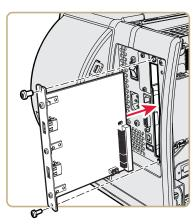
Use the T20 Torx screwdriver to secure the board assembly to the spacer screw with a Torx screw.
