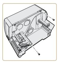
**2** Use a T20 Torx screwdriver to remove the two screws located on the outside of the electronics cover.
