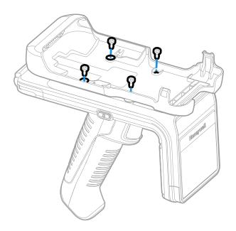
**Note:** The attachment screws ship with the bracket for the mobile computer. The screws are size M3x.5x6. Using a different size screw than those provided with the bracket may damage the RFID reader.
