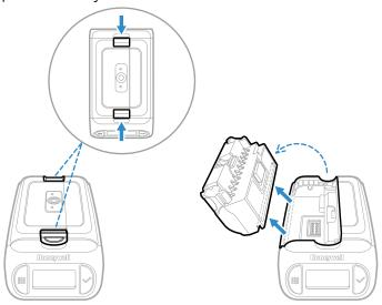
Replace the battery by aligning with the side of device and snapping it in to the device.
