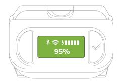
The window shows prompts for using the device in your environment. The buttons to the left and right of the window are used to scroll through the windows or to enter responses to screen prompts.
