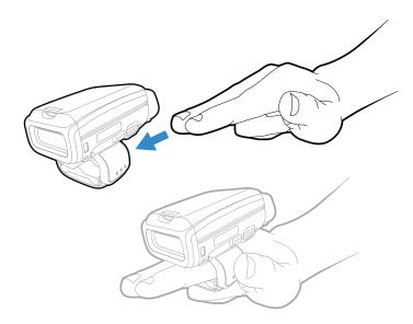
1. Press the free end through the loop and press the excess down to secure the strap.
