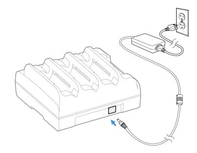
It is important that batteries are inserted into the charging pocket correctly. Inserting the battery incorrectly could result in damage to the battery or the charger.
