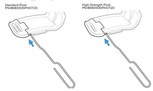
3. Slide the silver bar out and remove the old pivot.
