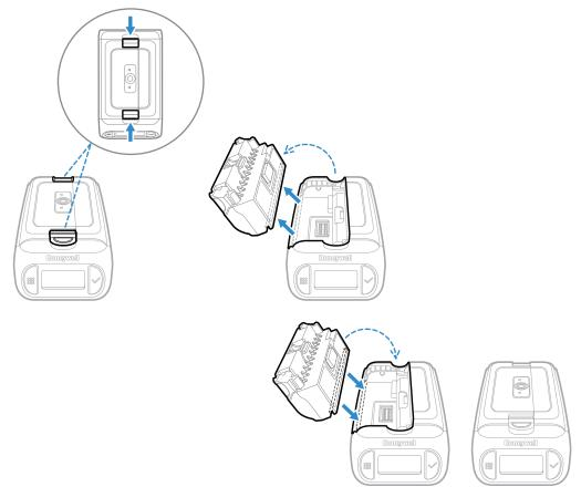
Replace the battery by snapping it in to the 8690i.
