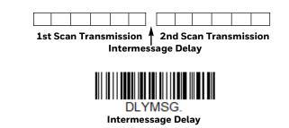
To remove this delay, scan the **Intermessage Delay** barcode, then set the number of delays to **0**. Scan the **Save** barcode from the Programming Chart, beginning on page 253.
