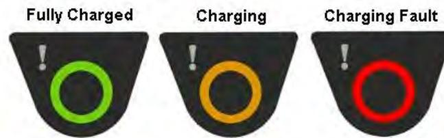
Figure 9: Battery Port Indicators
