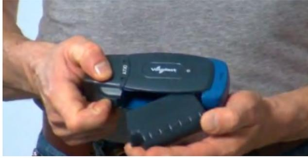
Figure 3: Removing the Battery From a Device
