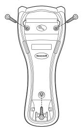
**Note:** Suitable for mounting at heights less than or equal to 2 m. (6.56 ft.)
