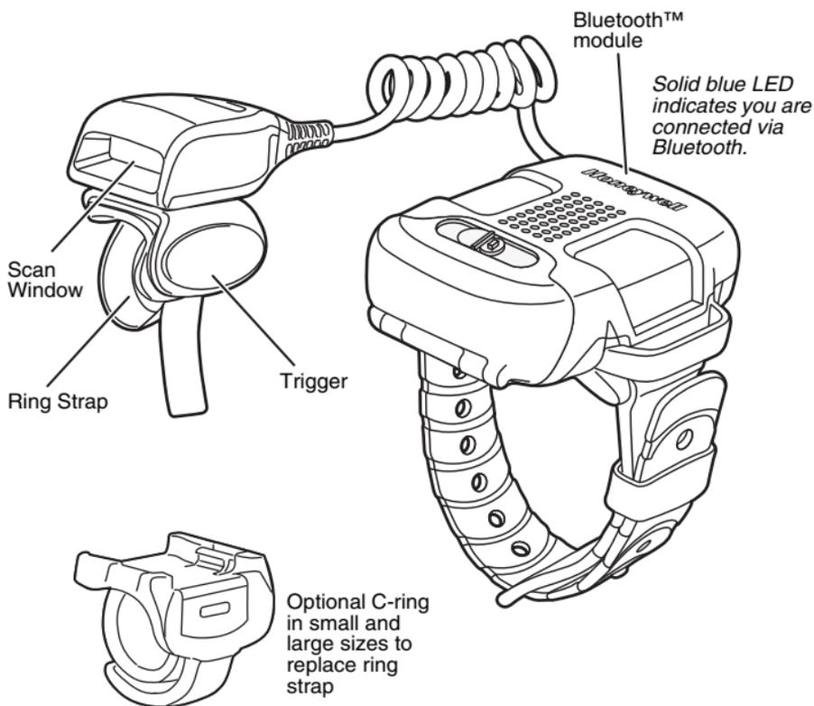
**Note:** *The battery must be fully charged before the first use. The 8650 8-Bay Battery Charger must be purchased separately.*
