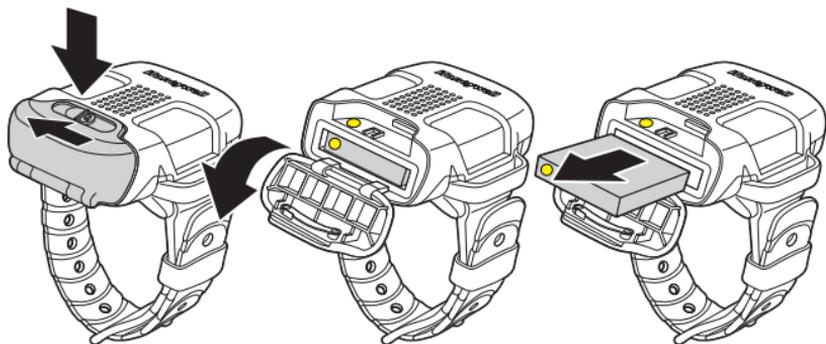
Replace the battery in the compartment, aligning the yellow dots on the battery and compartment, then slide the lock closed.
