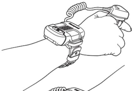
Right handed - wear battery module so Honeywell name is facing toward you
