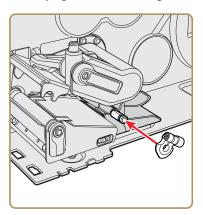
**11** Reconnect the label gap sensor cable and reinstall the upper media guide onto the media guide post.
