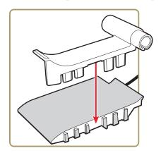
**8** Slide the coupler assembly onto the media guide post and feed the antenna cable through the hole in the printer base.
