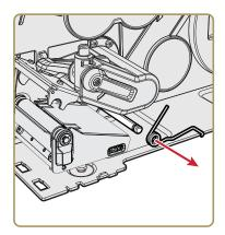
Attach the coupler holder to the coupler board assembly.
