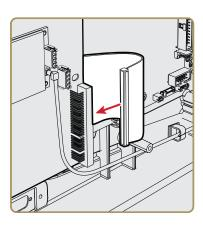
Use the 4-pin cable to connect the RFID board assembly to the RFID antenna on the assembly board.
