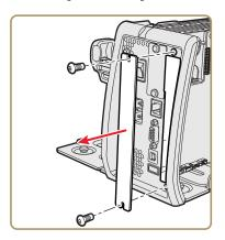
**2** Insert the RFID board assembly into the printer and use the T20 Torx screwdriver to secure the RFID board assembly to the spacer screw with a Torx screw.
