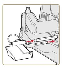
**9** Slide the media guide onto the media guide post with the flat side facing away from the media path.
