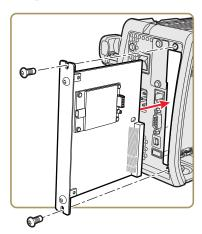
**3** Use the T20 Torx screwdriver to secure the RFID board assembly to the printer with two Torx screws.
