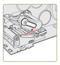
**2** Use a small slotted screwdriver to gently pry the upper media guide loose from the media guide post. Gently pull the upper media guide away from the printer until you can easily reach the label gap sensor cable.
