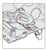
**10** Slide the media guide retainer onto the media guide post and secure it in place with the thumbscrew. Make sure it fits securely against the media guide.
