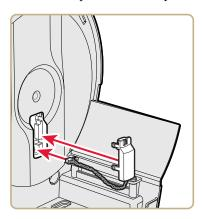
On the electronics side, connect the media sensor cable to the connector labeled "P26 Paper" on the main board.
