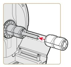
**10** Place the spring on the metal rod and secure to the rotation hanger with the Torx screw and metal washer. For best results, place the washer on the screw before inserting it into the metal rod.
