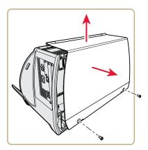
Remove the electronics cover, and put the cover aside on a soft cloth to avoid scratches.
