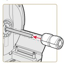
**9** Connect the second two 1 7/8-inch core pieces together and slide onto the metal rod. Make sure the alignment pins on the second set of core pieces line up with the alignment holes on the first set of core pieces.
