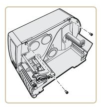
Use a T20 Torx screwdriver to remove the two screws located on the outside of the electronics cover.
