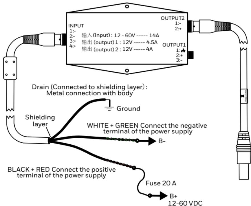
Determine the best method for connecting the power converter to the power source and for routing the cable, taking into consideration the following principles.
