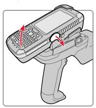
2. Remove the mobile computer hand strap from the locking bracket.
