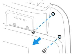
2. Attach the latch support using the  $M3 \times 12$  screws.
