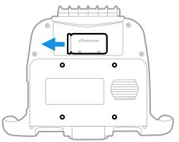
If the RT10-DOCK-RELEASE is installed (see page  $^{24}$ ), push the latch to release the clip.
