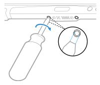
5. Ensure the inserts are flush with the tablet.
