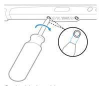
4. Ensure the inserts are flush with the tablet.
