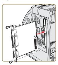
**4** Use the T20 Torx screwdriver to secure the interface board assembly to the spacer screw with a Torx screw.
