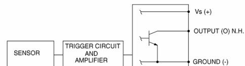
**ELECTRICAL SPECIFICATIONS** over 3.8 Vdc to 30 Vdc and -40 °C to 150 °C [-40 °F to 302 °F]
