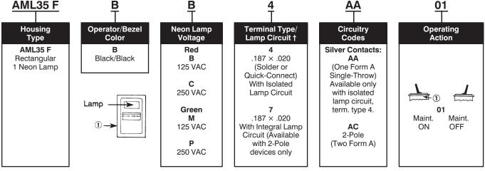
1) The "MICRO SWITCH" identification is shown on this side of the switch housing.
