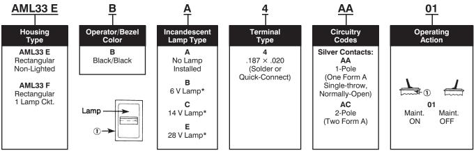
\* Lamps will be installed per each lamp circuit specified in the Housing Type.
