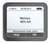
Once the internal memory is 95% full (9,499 measurements), a "Memory 95% full" message appears in the display.
