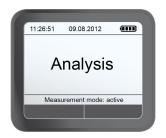
The yellow LED is flashing during the evaluation of the breath sample. Depending on the alcohol concentration this can take several seconds. Device indicates end of the analysis with a single audible signal.
