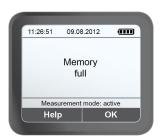
After the 9,999th measurement, the message "Memory full" appears on the display. If any further measurements are taken, a query appears asking whether old data should be overwritten. This has to be confirmed once by pressing >YES< or >NO< and does not appear again until the device is restarted.
