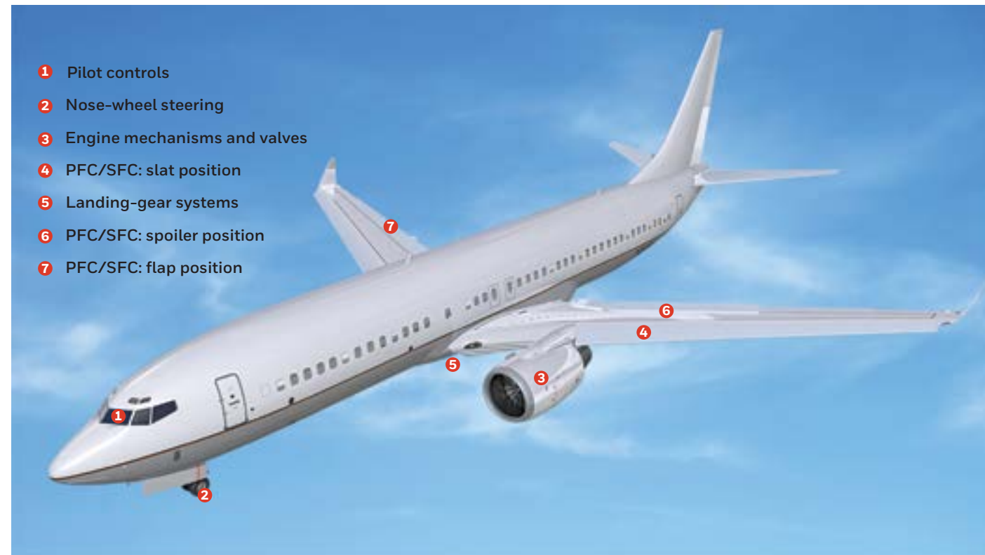
Figure 1. LVDT Position Measurement Applications for Aircraft
