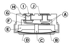
A ContactsF Contact armB Bimetal discG Metal sleeve (3004 only)C Ceramic transfer pinH Phenolic baseD Metal closureI Rivet (3004 only)E Phenolic insulatorJ Terminal
