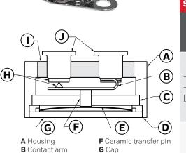
**B** Contact arm **C** Ceramic insulator **D** Laser weld E Bimetal disc
