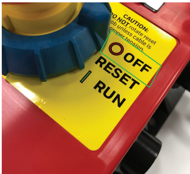
FIGURE 4. 2CCP WITH BLUE RESET KNOB IN OFF POSITION
