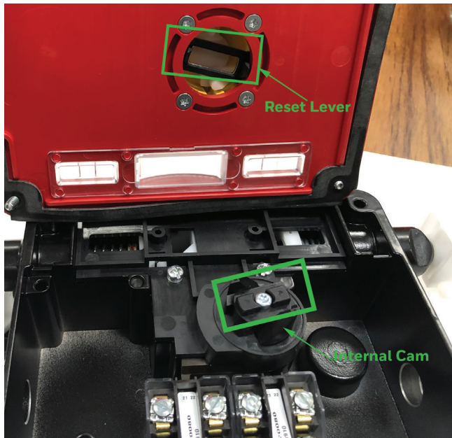
FIGURE 3. RESET KNOB/LEVER AND INTERNAL CAM
