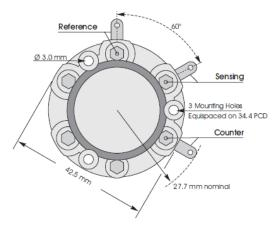
All dimensions in mm All tolerances ±0.15 mm unless otherwise stated 3ND shown with side tags and tin pins
