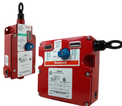
Each CPS switch has travel specifications. The distance between “trip on slack” and “trip on pull” is the usable travel. The lesser the travel, the lower the temperature tolerance a CPS will have. With 0 °C [0 °F] change in temperature, only the weight and friction of the cable are factors in its correct operation and very long runs are theoretically possible. Real world applications have temperature variations for which planning is needed.
