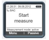
After switch-on the device operates automatically in the active mode and the Display shows "Start Measure".
