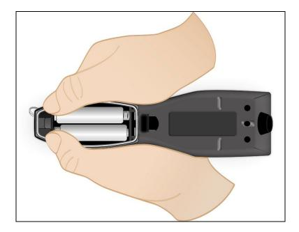
The battery compartment holds a battery block with 4x LR6 (AA) alkaline Mignon batteries (Industrial by Duracell recommended). As a general rule, all four batteries should be replaced at the same time. Ensure the polarity of the batteries is correct. The battery block is then reinserted into the case. The battery block connections (arrow) must face towards the device and be on top as shown in the following image. The battery compartment cover can now be closed again.
