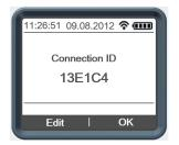
Having selected the option >Wireless<, an appropriate wireless printer can be used. Prior to the initial wireless operation, the printer and the AlcoQuant 6020 plus need to be paired with each other by using the Connection ID of the printer. The single digits of the printer Connection ID have to be set with the key >Edit<. Finally confirm the Connection ID with >OK<. A printer test can then be performed with >Print<.
