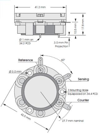
ELECTRICAL Recommended Load Resistor 33 Ω Bias Voltage Not Required
