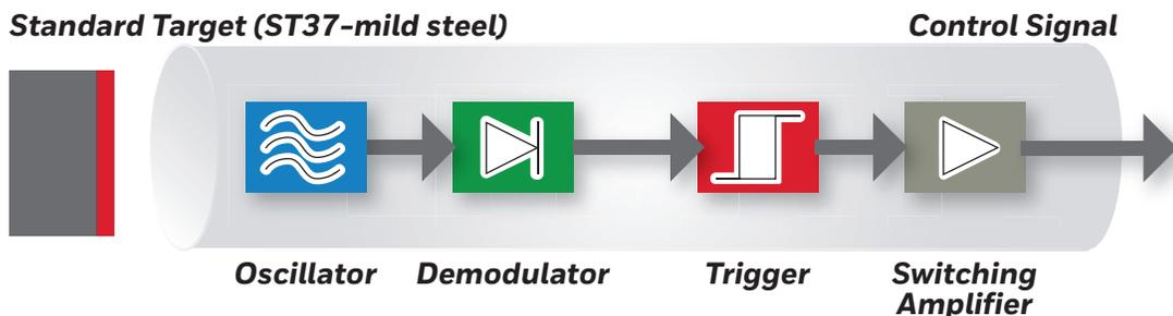
Honeywell has enhanced the existing technology to offer a next-generation Series of proximity sensors.
