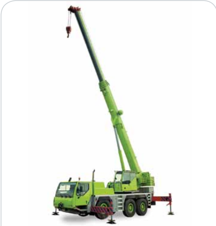
Figure 10. Truck mounted crane outrigger position
