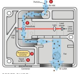
Engineered for excellent accuracy, the HPM Series employs a laser-based sensing approach that detects airborne particulates with incredible accuracy.
