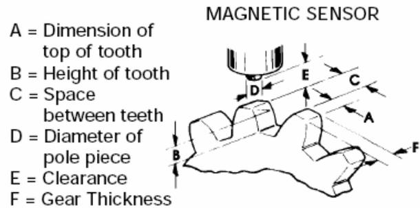
The above configuration is usually not available in a stock gear, but it is seldom necessary to have the maximum output. Very close to the maximum output may be generated by conventional stock gears if the tooth width **A** is equal to or greater than the pole piece diameter and **C** is 1.5 times **D**.
