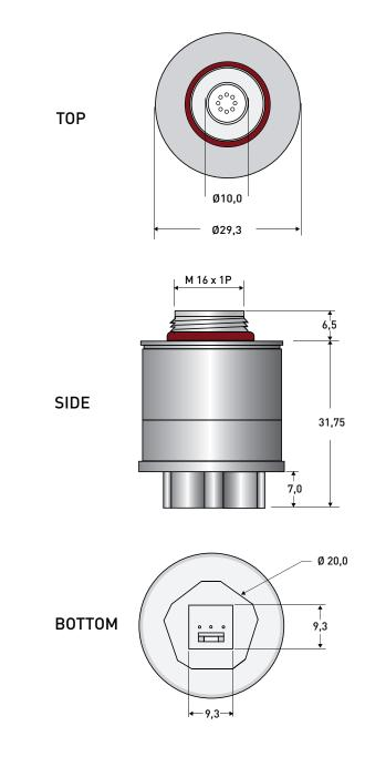
**Important Note:** Connection should be made via recommended mating parts only. Soldering to the sensor will damage it and invalidate the warranty.
