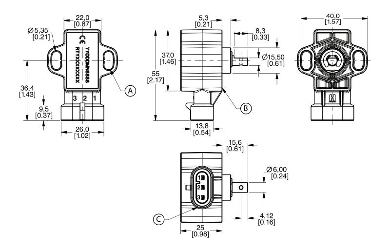
Mount sensor with non-magnetic stainless steel M5 screws. Mounting torque is  $2,5 \pm 0,5$  N m [ $22.1 \pm 4.4$  in-lb].
