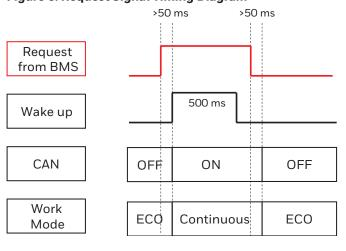
5.3.2 Wake-up Signal Set to High: The BPS sets its Wake-up signal to high when in ECO mode and the absolute pressure or rate of change of pressure in the battery pack is above the configured threshold.
